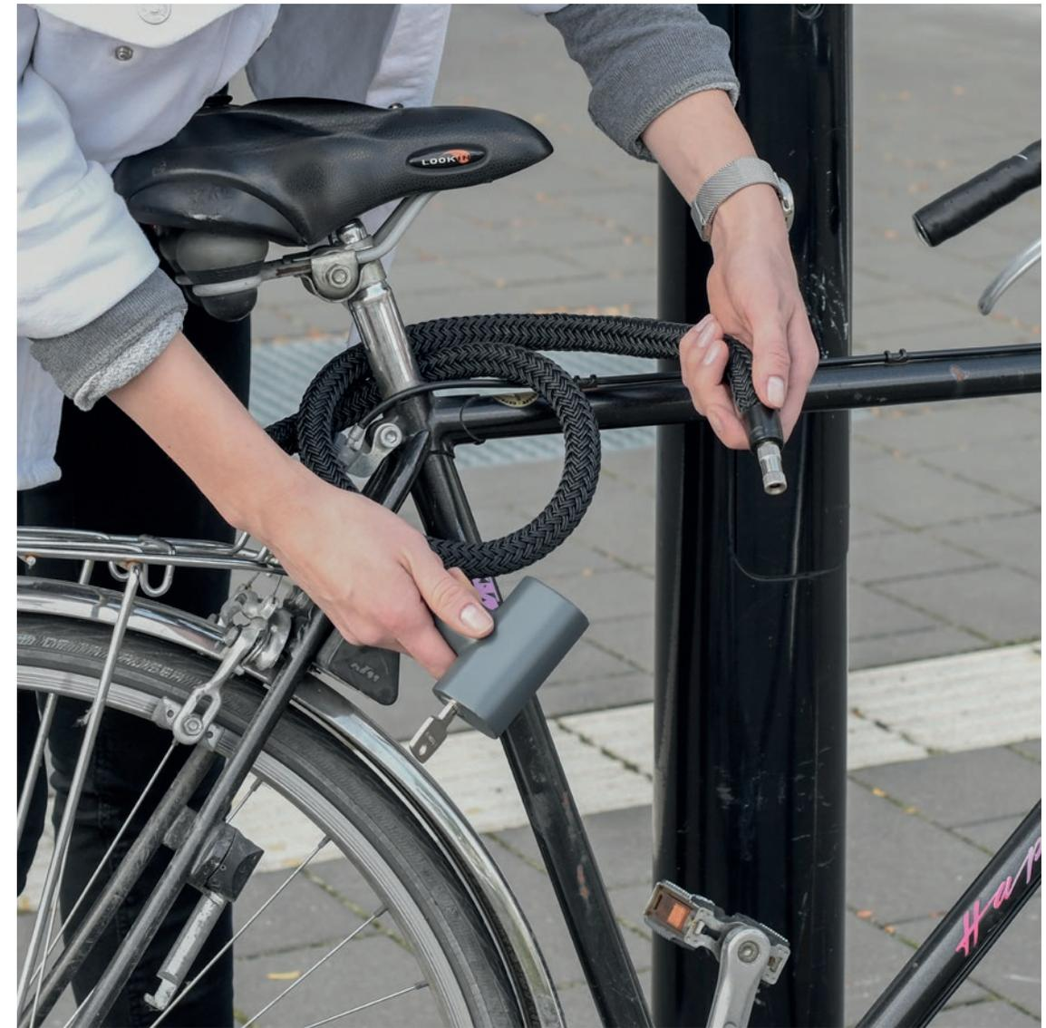
*Due to the length of the hose and its flexibility, an ergonomic posture can be adopted during pumping. The valve also serves as the lock's closing mechanism, which converges into the pump's handle.*
